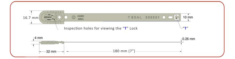
The Metal T Seal has inspection holes for ensuring seal is properly locked and not pre-tampered.
